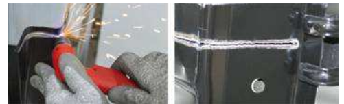
STEEL : 10 mm max ALU : 8 mm max (Speed = 9 cm /min at 30A)
