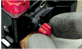
Adjustment of the rivet setting speed
