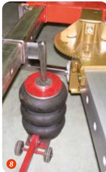
Pneumatic lift that belongs to B5 basic set makes mounting of a vehicle easy. The collision repair system can easily be lifted to a suitable ergonomic working height with help of the pneumatic lift.
