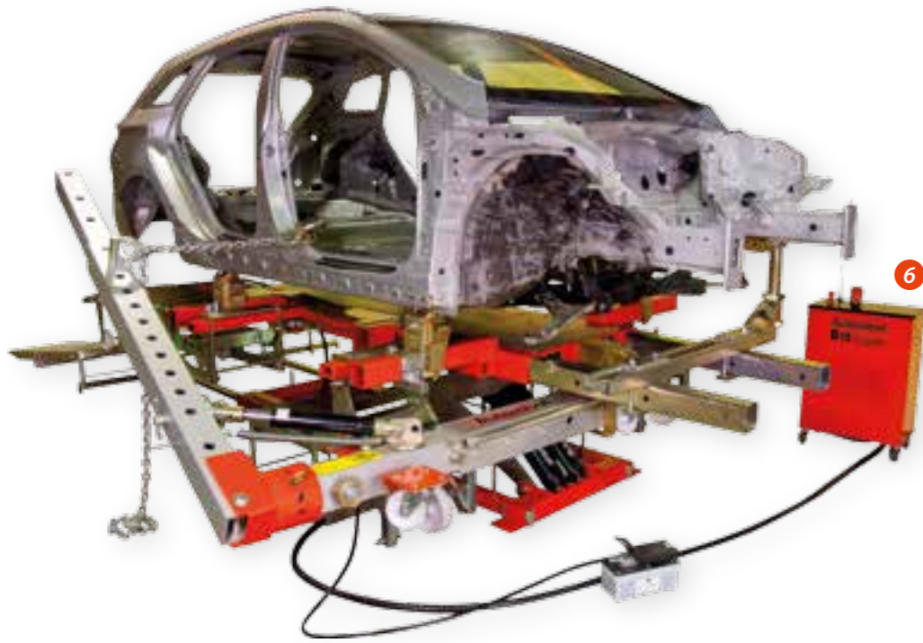
Autorobot B15 Super is equipped with electric hydraulics that is controlled from the remote-control panel (picture 6). Picture 7 shows the upward pull of the box section under the control of electronic measuring.
