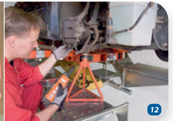
Picture 12: Installing new ball joint by using B15 lift/lowering technique.
